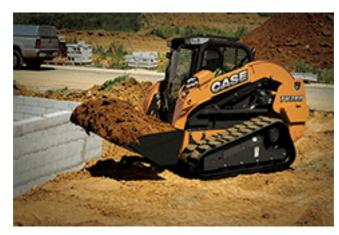
an arc, this configuration provides greater reach at mid-ranges, which makes it ideal for loading and unloading off of smaller vehicles or platforms, such as pick-up trucks. Visibility also tends to be a bit better with radial configurations.
