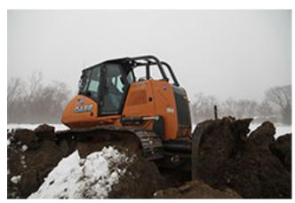
Undercarriage maintenance and upkeep is not a short-term effort. The only a time a machine's undercarriage is not experiencing wear is when it's standing still – and machines that stand still don't make money. The undercarriage also represents a high percentage of the total operating cost of the machine over its life. With dozers, approximately 20 percent of the purchase price and 50 percent of the maintenance cost sits in its undercarriage.
